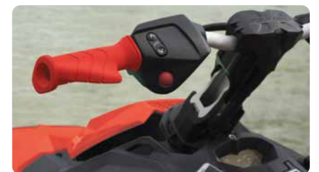
Extended Range VTS™ (Variable Trim System) Offers double the range of the regular VTS™ for greater ease when executing tricks.
